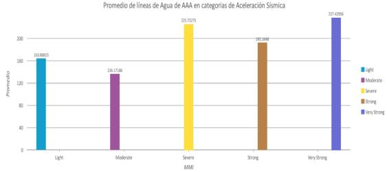
Figure 3-67. PRASA water lines exposed to seismic acceleration.
