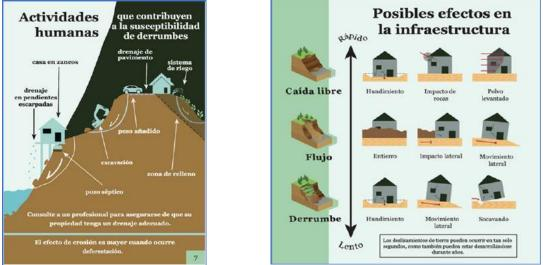
**Figure 3-2.** Human activities contributing to landslides. Source: USGS, UPRM, Natural Hazards Center, 2020. **Figure 3-3.** Possible effects of slip types on infrastructure. Source: USGS, UPRM, Natural Hazards Center, 2020
