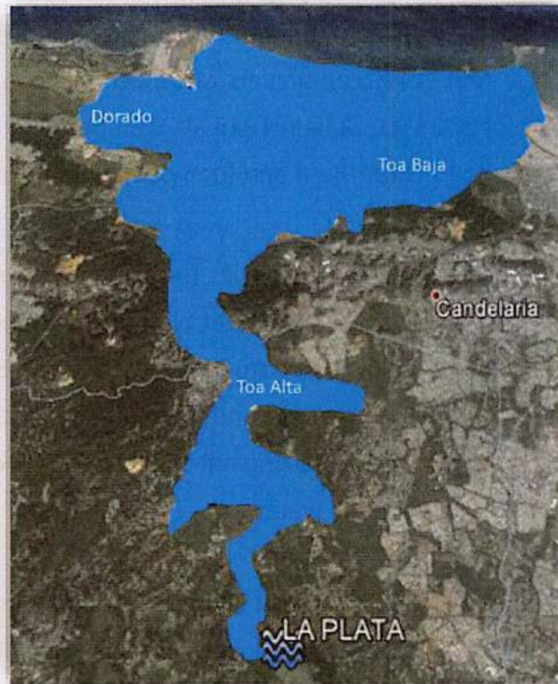
Collapse Flood Map of the Silver Dam in Toa Alta 29 18.343259, -66.236069
