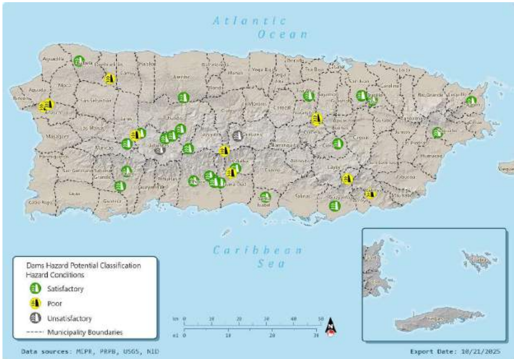
Figure 315: Qualitative Classification of Dam Conditions in Puerto Rico, Based on Secondary Information
