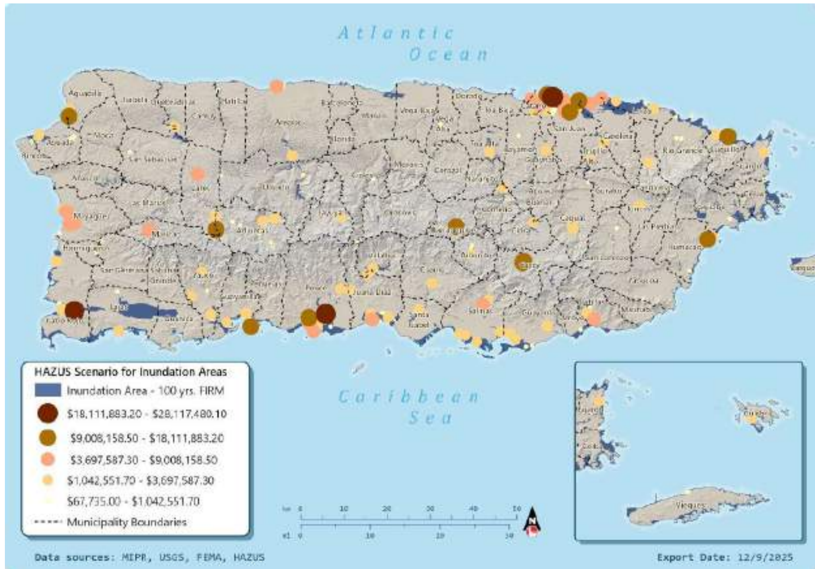
Figure 165: Estimated Critical Infrastructure Replacement Value in Puerto Rico's 100-Year Floodplain (FIRM Scenario)
